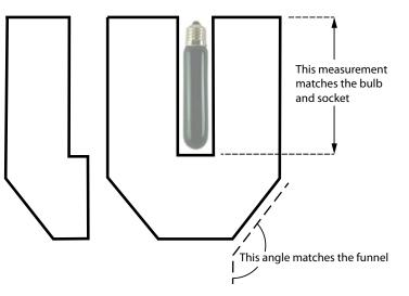
On the centre line of the U' shaped baffle, cut halfway through, then slip the edge of the single baffle into the opening created.
