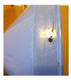
Drill three 3mm holes in the funnel edge close to the top rib, spaced at 120 degrees. (Use the baffle assembly rig to mark the spacing.)
